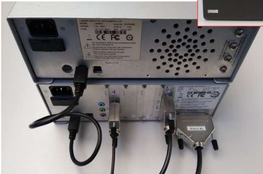
Optional LNP connected via the Instrument bus cable
